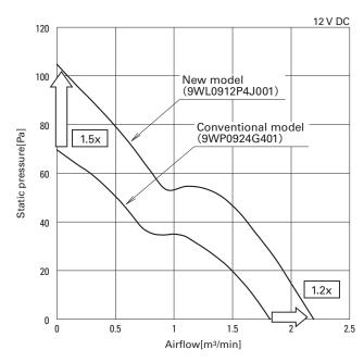
Fig. 10: Airflow vs. static pressure characteristics of "San Ace 92W" New/conventional model comparison
