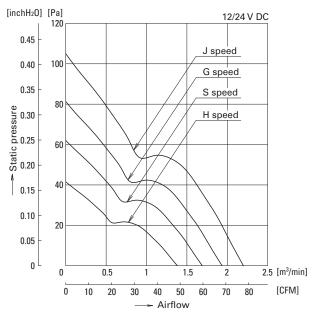
Fig. 7: Airflow vs. static pressure characteristics of "San Ace 92W"
