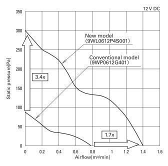
Fig. 8: Airflow vs. static pressure characteristics of "San Ace 60W"New/conventional model comparison
