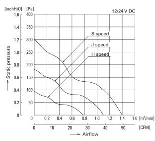
Fig. 5: Airflow vs. static pressure characteristics of "San Ace 60W"
