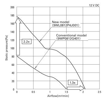
Fig. 9: Airflow vs. static pressure characteristics of "San Ace 80W" New/conventional model comparison
